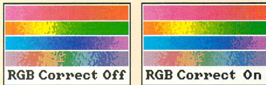
Figure 3. If a standard printout (left) does not match your screen colors, turn on Color Correct R/G/B (right).
