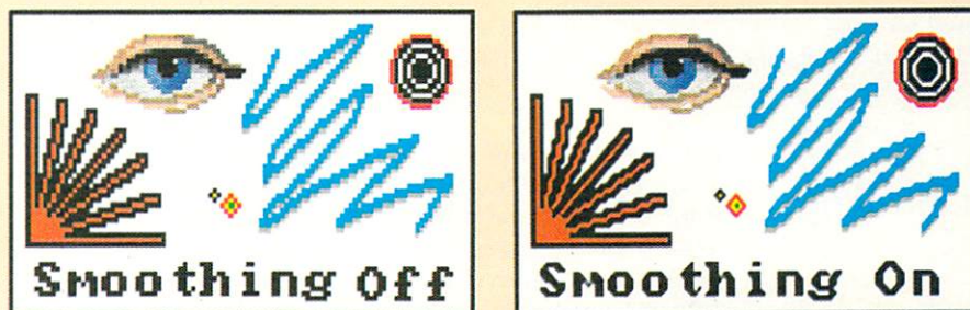
Figure 2. With Smoothing off (left) diagonal lines and curves are jagged. Smoothing On (right) softens the effect.
